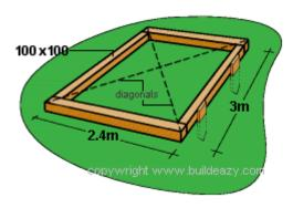
Once the level greenhouse site has been determined, make the base, constructed out of 100x100 tanalised h4 sawn timber. This timber is readily available at any timber merchants and commonly used for fence posts. Standard lengths are 2400mm and 3000mm.
