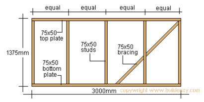
On a flat piece of ground, make two side walls up as per dimensions shown in the drawing above.
