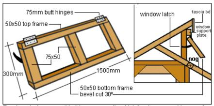
For the windows use 50x50 sawn tanalised h3 for the top and bottom frames and 75x50 sawn tanalised h3 for the side and middle mullions.
