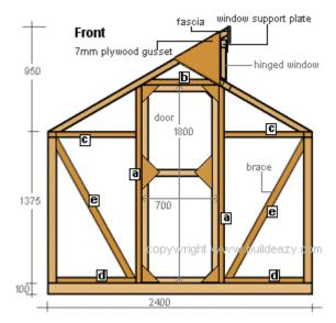
Ensure side walls are plumb (vertical)
