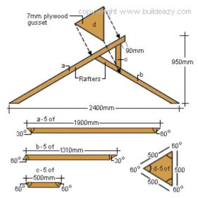
Cut all roof frame pieces as per dimensions shown above. Use 75x50 tanalised h3 sawn timber.
